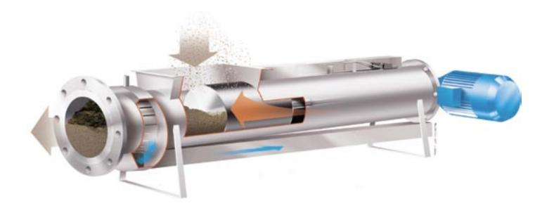
Roto-Sieve piston presses from Läckeby Products combine the good dewatering capacity of a screw press with the capability of a hydraulic press to lift and transport the dewatered material. This is made possible by the drive system's flexibility.
