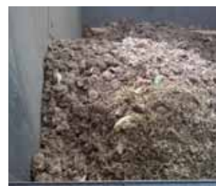
The grit from a WSP press contains higher amount of dry solids - over 50 %.
